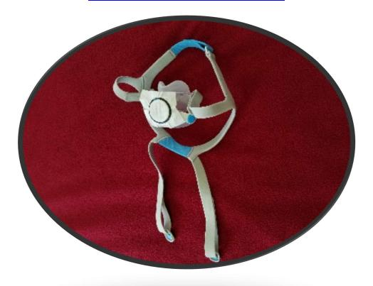
ABOVE IS A HOMEADE DEVICE USING A CPAP MASK. THIS TYPE COVERS THE NOSE AND MOUTH (NOT ALL OF THEM DO SO). USING A FILTER FABRIC MADE BY 3M FOR HVAC **DEVICES WITH A MERV (HVAC FILTER RATING SYSTEM) 12** RATING: 1.0 – 3.0 μm @ >95% EFFICIENCY. YOU MAY FIND A HIGHER MERV FILTER FABRIC OR YOU COULD DOUBLE IT UP BUT IT WILL BE VERY HARD TO BREATH THROUGH SUCH A SMALL OPENING.
