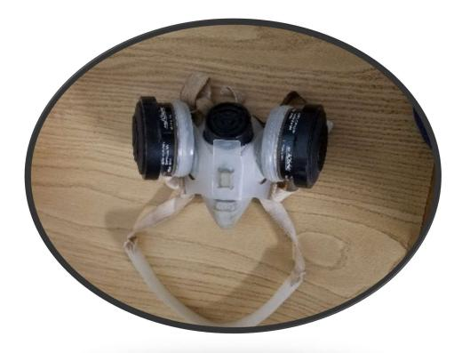
ABOVE IS AN INDUSTRIAL MASK (TYPICALLY REFERRED TO AS AN ELASTORMERIC RESPIRATOR). THE FILTERS VARY DEPENDING ON THE TOXINS / PARTICULATE MATTER YOU WANT TO KEEP OUT OF YOUR LUNGS. CAN BE VERY EFFECTIVE BUT YOU ARE NOT GOING TO WANT TO WEAR FOR VERY LONG AS THEY ARE HEAVY, HOT, HUMID, AND UNCOMFORTABLE.
